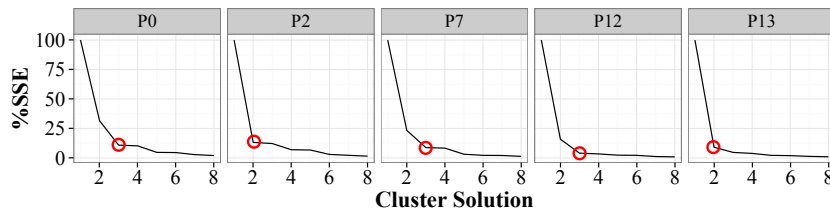
Figure 11: Elbow plot for determining the best number of clusters for the Intel i7 server power model. The circles highlights the number of clusters chosen to partition the data set.
